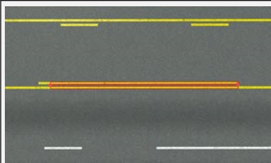
Span selected in the Lane Marking Tool . This span defines the lane marking type between two nodes.
