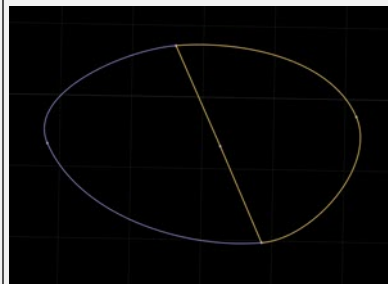
Region is automatically split into two regions when two closed loops are formed.
